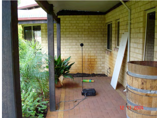
Figure 3.1 – Automatic Noise Data Logger
